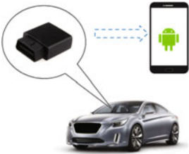
Fig. 3 Data collection schematic using the OBD interface and smartphone
