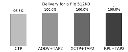
Figure 4. Transferring a 512KB file to a node 5 hops away from the root.
